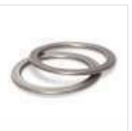
Metal Jacketed Gaskets with a compressible insert that makes the gasket suit the flange. Metal jacketed gaskets can be made with a broad range of metals and high temperature fillers.
