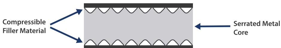
Expanded graphite is the most common facing material used for our Kammprofile gaskets. However, other materials can be used, such as PTFE for chemically aggressive duties or mica for high temperature service.
