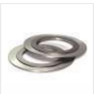
The Kammprofile is a Grooved, covered metal gaskets consisting of a serrated metallic core with a soft facing material.
